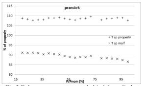
Fig.3 Exhaust gas temperature behind the cylinder recognized as properly (Tsp properly) and behind the cylinder with the leakage of the fuel injection pump (Tsp malf)
