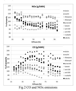
According to presented results, simulated engine malfunction cause a change in the organization of the combustion process in engine cylinders. The result is a change in fractions of chemical compounds in the exhaust gas. For example, the throttling of the exhaust gas duct, causes up to 80% increase of the CO fraction in the exhaust gas.
